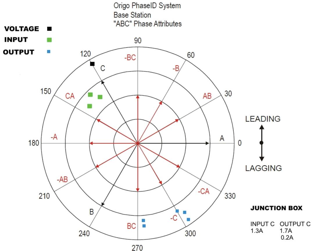
The black square is the voltage phase measured on the input elbow capacitive test point. The green squares are from multiple current phase measurements on the same elbow. Note that the current phase is nearly in phase with the voltage.
