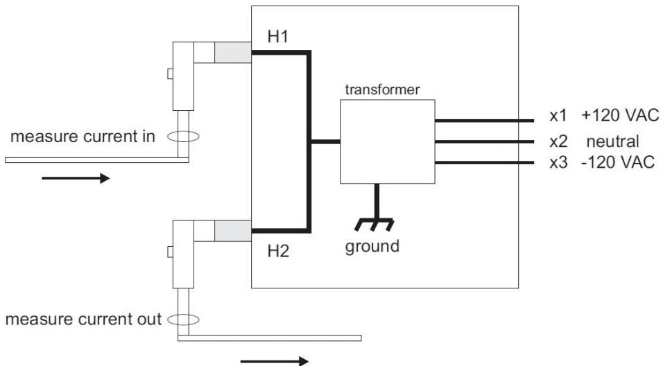
Inside the padmount, bushing H1 and H2 are connected together and to the transformer, which converts the URD 7200 VAC power to 120 VAC residential power. Incoming power from the upstream padmount is connected to H1 while H2 provides power to the remaining downstream padmounts. The fact that both bushings (and both elbows) are connected together, prevents the use of a line locator from determining
