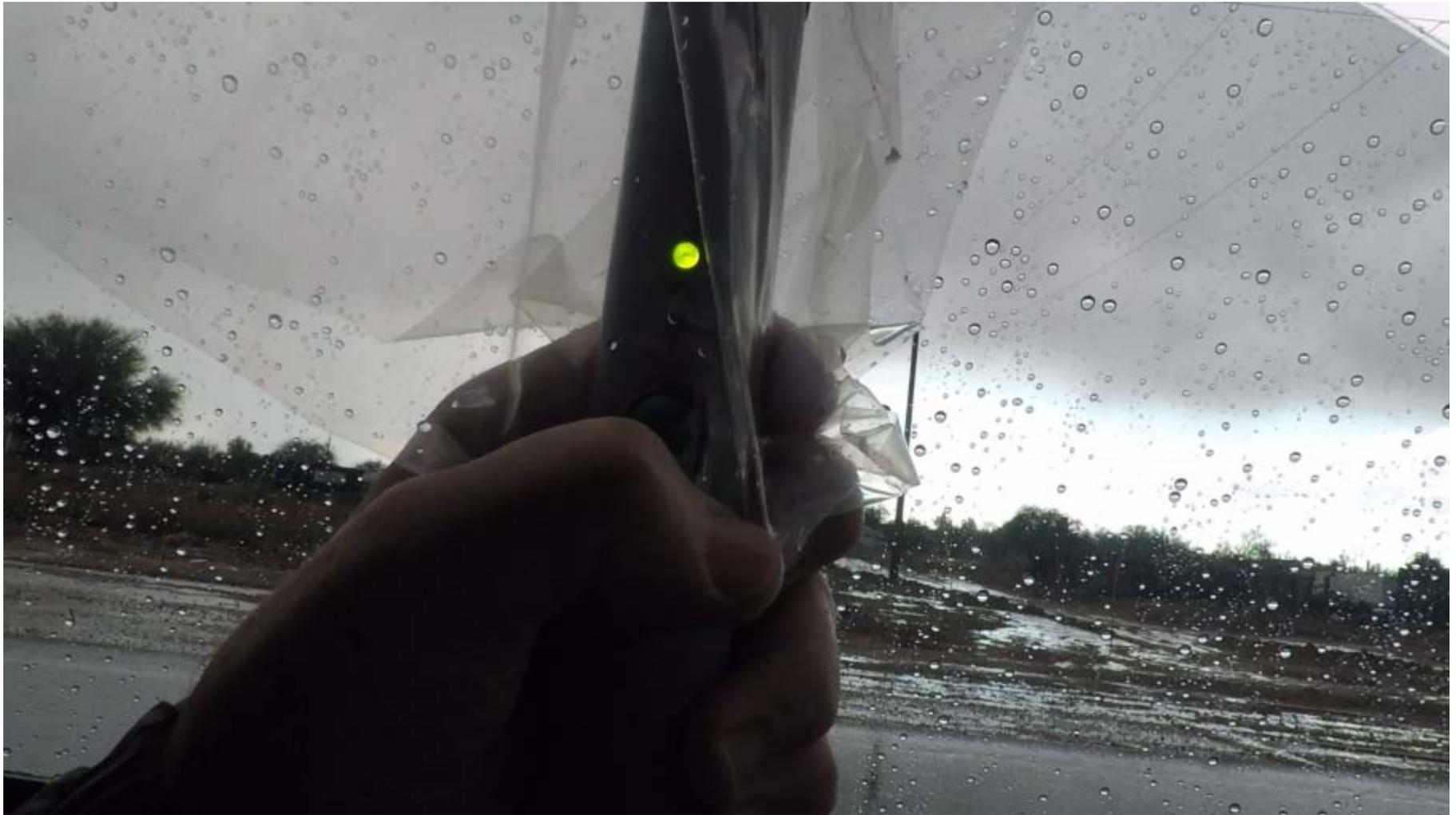
**Attach the probe to an extendo stick in crowded circuit situations like underbuild**
