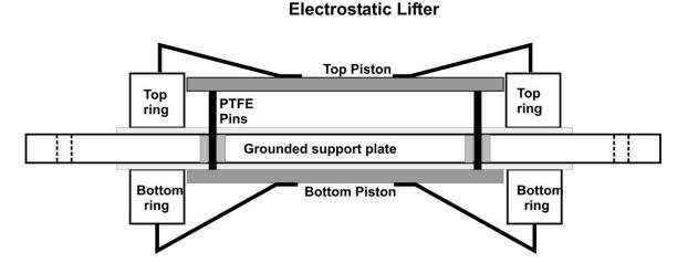
When a high voltage is applied to the top piston via the top ring and spring clips, an electrostatic force of attraction is produced between the top piston and the grounded support plate.
