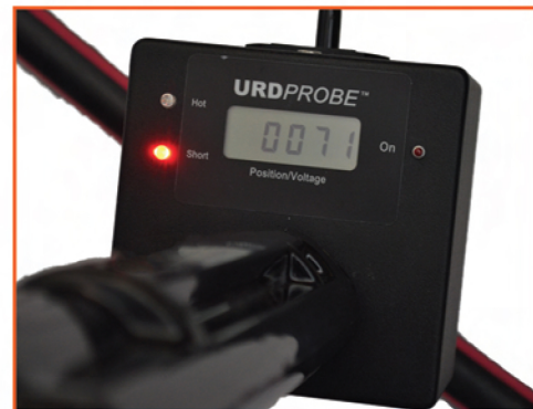
Red LED indicates needle short to concentric.
