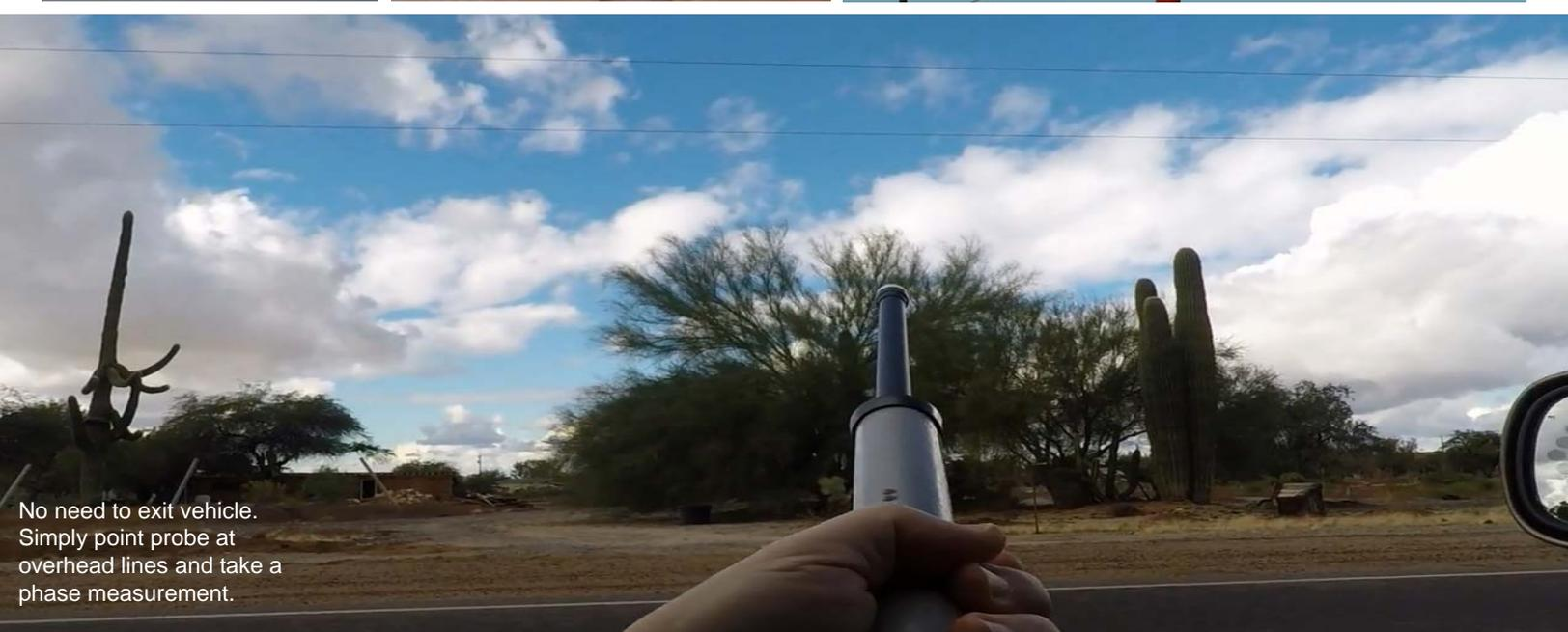
No need to exit vehicle. Simply point probe at overhead lines and take a phase measurement.
