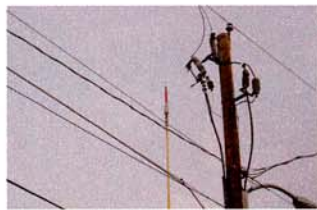
The field probe (attached to the end of a telescoping hotstick) gathers overhead phase data by touching the conductor.
