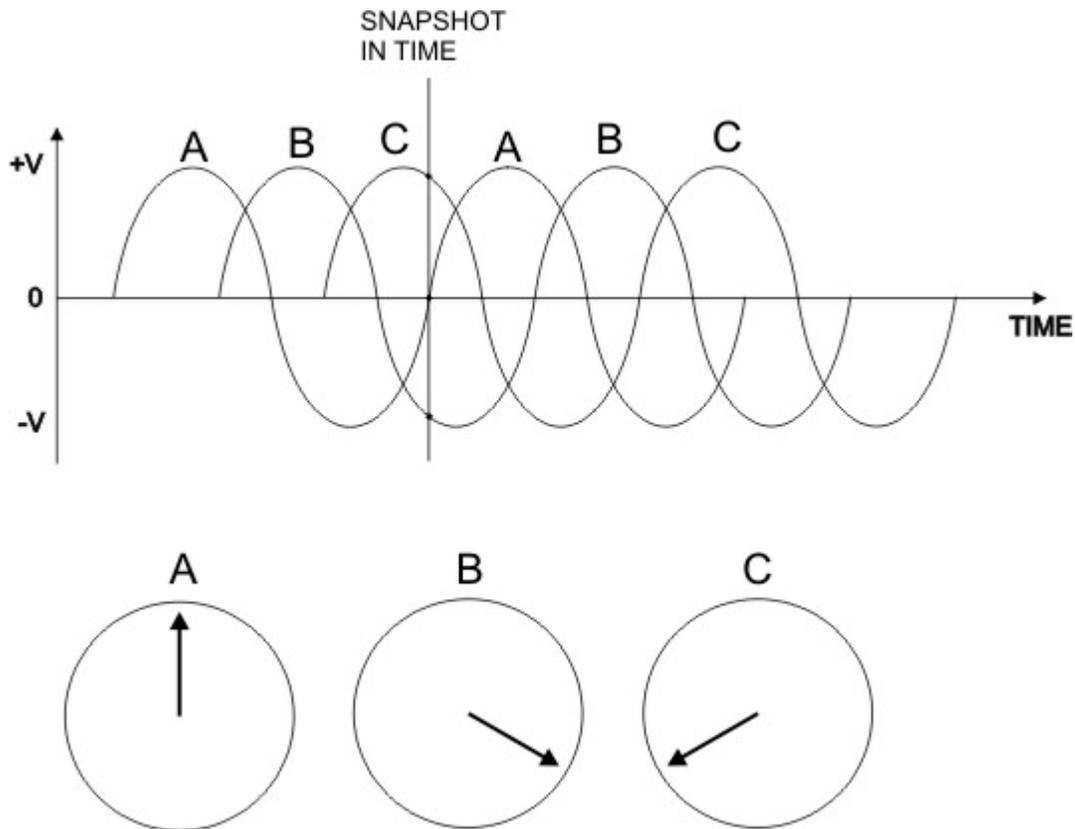
Therefore, if it was known that the reference motor was connected to phase “B”, the phase to which a second similar motor was connected could be determined simply by noting the relative orientations of the second motor arrow with respect to the reference motor arrow.
